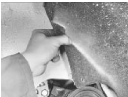
10.4B Removing wing shield
