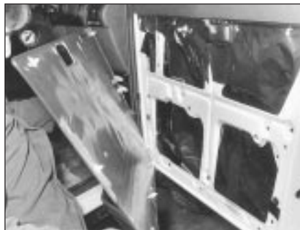
11.6 Removing door trim panel
