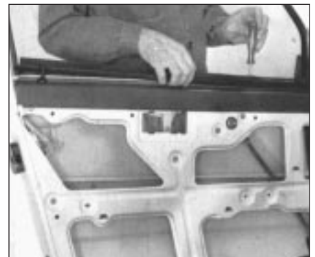
Fig. 12.7 Removing door weatherseal (Sec 12)
