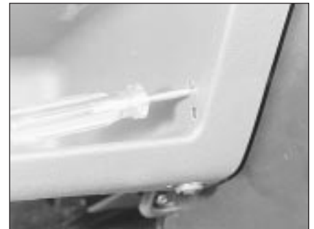
21.3 Removing screw (glovebox side) from centre console
