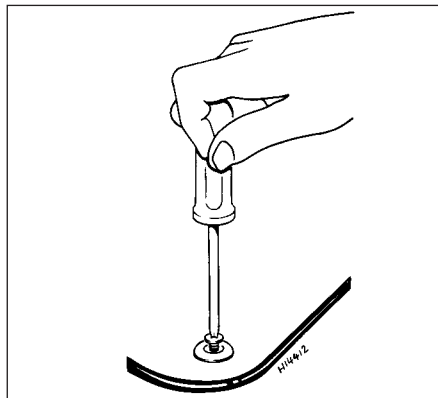
Fig. 12.25 Extracting sunroof panel screw (Sec 28)
